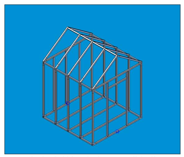
ABOVE DISPLAY IS AN 8X8 PORTABLE STEEL SHED FRAME WITH FLOOR STRUTS ON 2' FT CENTER SPACING USING QUICK BUILD CONNECTORS - 3' DOOR IS PLACED IN SHORT WALL (configuration of steel may vary due to production constraints - frames-black - display colors0 4 affect)
